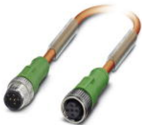
Sensor/actuator cable, 5-position, PUR halogen-free, irradiated, orange RAL 2003, Plug straight M12, A-coded, on Socket straight M12, A-coded, cable length: 1 m, Customer version
