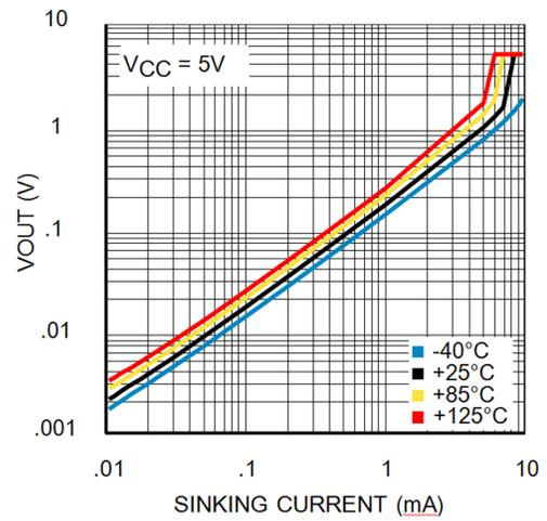
Figure 14. Saturated Output Sinking Current at 4.5 V
