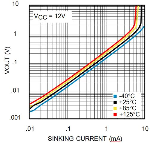
Figure 16. Saturated Output Current Sinking at 12 V
