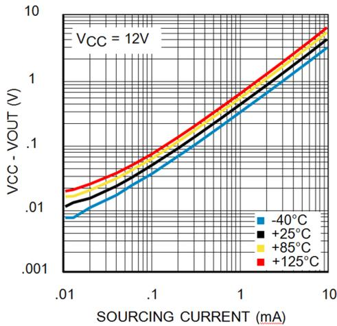
Figure 15. Saturated Output Sourcing Current at 12 V
