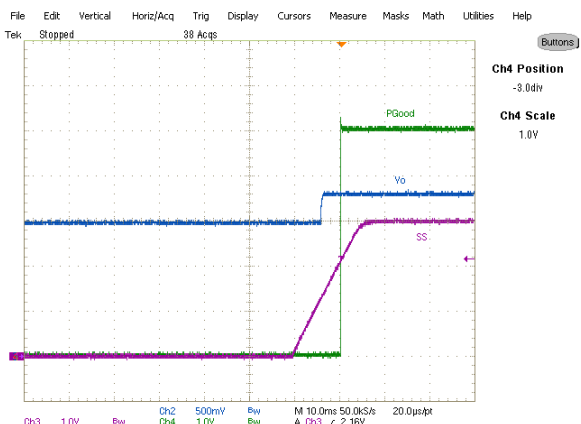
Fig. 23: Start up with 1.5V Prebias, 0A Load, Ch 2 :V out Ch 3 :V SS Ch 4 : PGood
