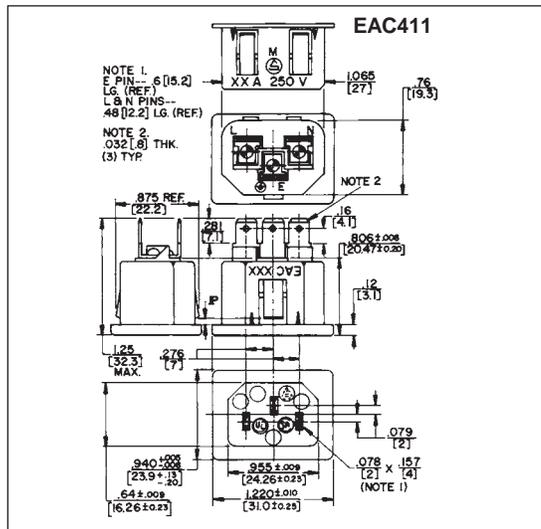
DIMENSIONS ARE FOR REFERENCE ONLY  $\frac{\text{Inch}}{\text{(mm)}}$
