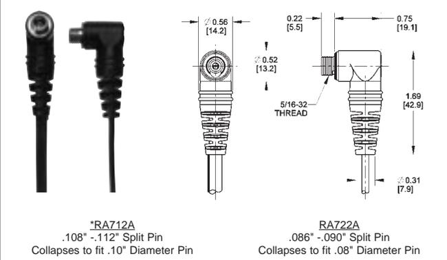
DIMENSIONS ARE FOR REFERENCE ONLY  $\frac{\text{Inch}}{(\text{mm})}$
