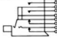
Double closed circuit. Isolated switching—Two "make" circuits.
