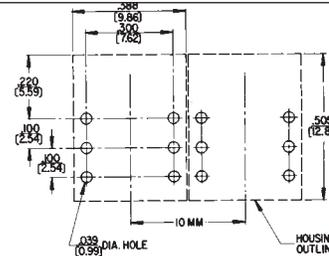
**RECOMMENDED PC BOARD LAYOUT (Component Side)**
