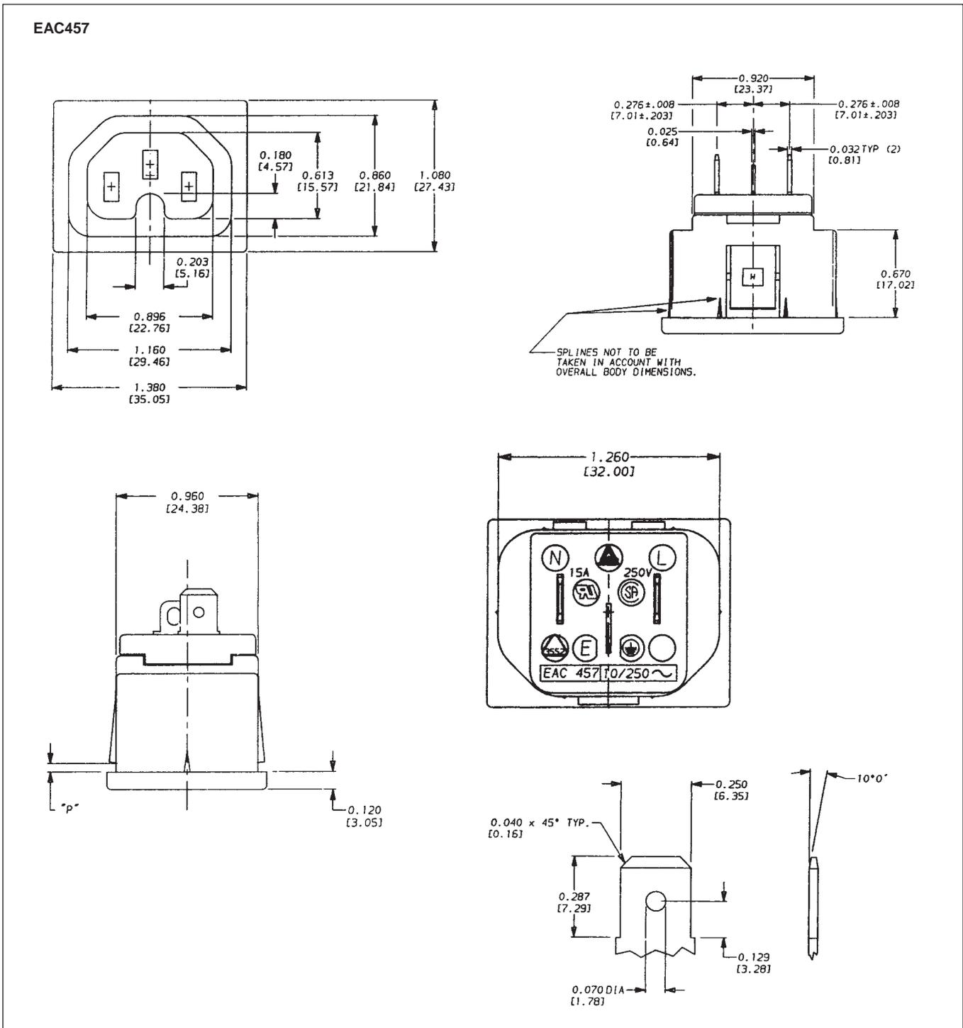
DIMENSIONS ARE FOR REFERENCE ONLY  $\frac{\text{Inch}}{\text{(mm)}}$
