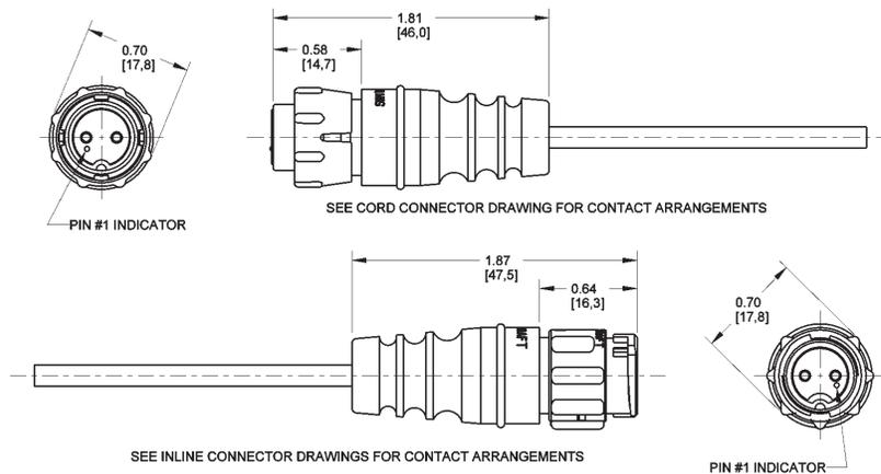
DIMENSIONS ARE FOR REFERENCE ONLY  $\frac{\text{Inch}}{\text{(mm)}}$
