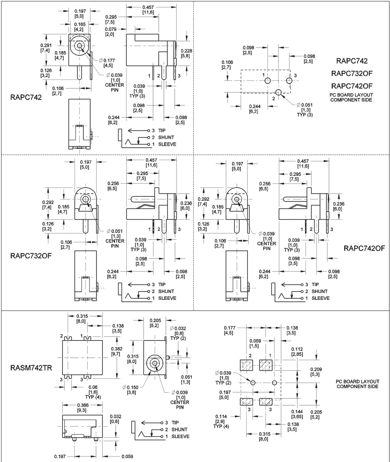
DIMENSIONS ARE FOR REFERENCE ONLY  $\frac{\text{Inch}}{\text{(mm)}}$
