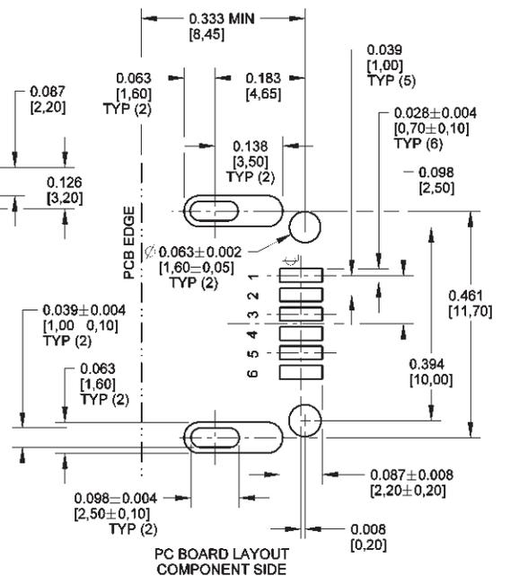
DIMENSIONS ARE FOR REFERENCE ONLY  $\frac{\text{Inch}}{\text{(mm)}}$
