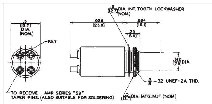
DIMENSIONS ARE FOR REFERENCE ONLY  $\frac{\text{Inch}}{\text{(mm)}}$
