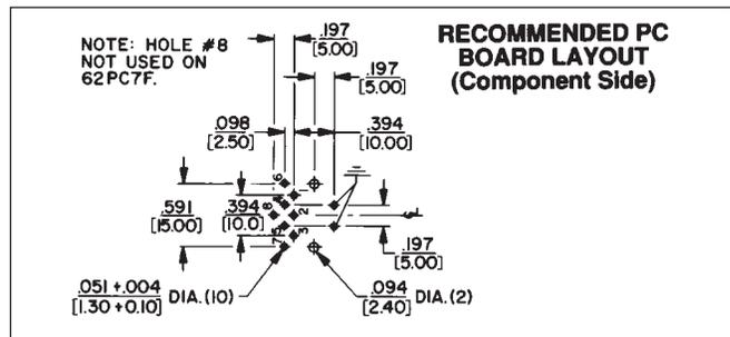
DIMENSIONS ARE FOR REFERENCE ONLY  $\frac{\text{Inch}}{\text{(mm)}}$
