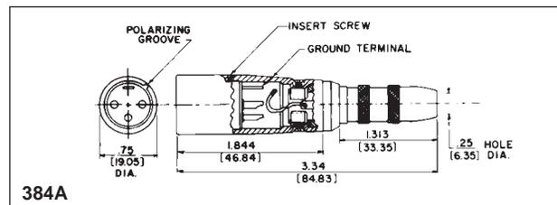
DIMENSIONS ARE FOR REFERENCE ONLY  $\frac{\text{Inch}}{\text{(mm)}}$
