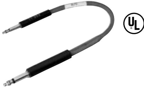
Series CPC Combination Patch Cords provide convenient interconnections between standard telephone-type jacks (3-conductor, .25" inside diameter sleeve) and miniature telephone-type jacks (3-conductor, .173" inside diameter). Series CPC cords are ideal for connection in telephone, data processing and other telecommunication applications where both standard and miniature jacks are available for patching.
