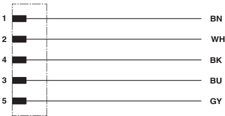
Contact assignment of the M12 socket
