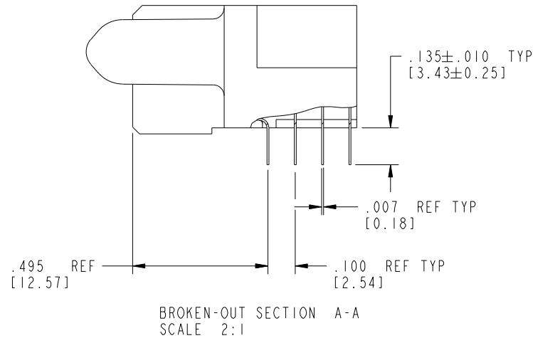
BROKEN-OUT SECTION A-A
