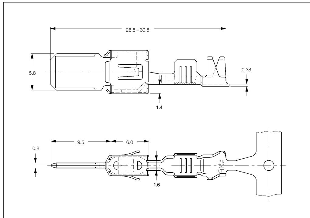
**Tab Contacts Single Wire Sealing System (SWS)**
