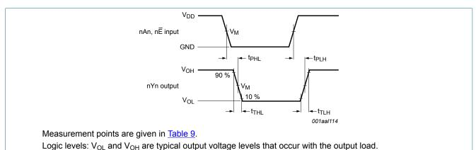
Inputs nAn, nE to output nYn propagation delay and nYn output transition time Fig. 4.
