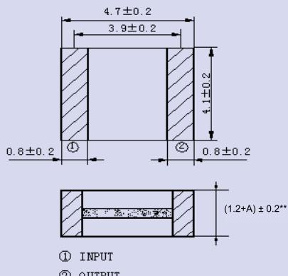
\*\* A stands for the thickness of the ceramic element, which varies with the frequency
