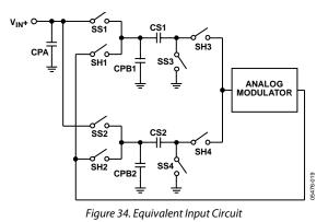
The AD7763 employs a double sampling front end, as shown in Figure 34. For simplicity, only the equivalent input circuit for  $V_{IN}$ + is shown. The equivalent input circuitry for  $V_{IN}$ - is the same.
