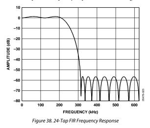
The coefficients for the filter in Table 14 are shown from the center of symmetry outward; that is, Coefficient 1 is the coefficient at the center of symmetry. The raw coefficients were generated using a commercial filter design tool and scaled appropriately so their sum equals 67108863 (0x3FF FFFF).
