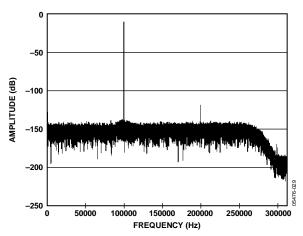
Figure 16. Low Power FFT, 100 kHz, –6 dB Input Tone, 32× Decimation
