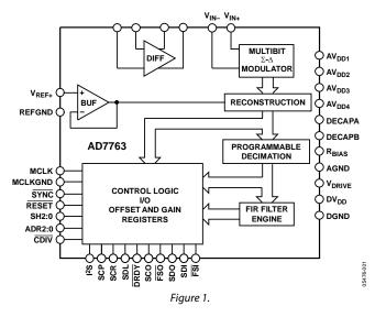
The differential input is sampled at up to 40 MSPS by an analog modulator. The modulator output is processed by a series of low-pass filters, the final filter having default or user-programmable coefficients. The sample rate, filter corner frequencies, and output word rate are set by a combination of the external clock frequency and the configuration registers of the AD7763.
