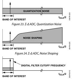
Figure 25.  $\Sigma$ - $\Delta$  ADC, Digital Filter Cutoff Frequency
