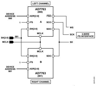
Figure 27. Two AD7763 Devices Operating Using the I<sup>2</sup>S Interface
