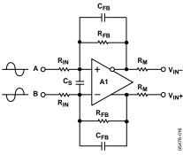
Figure 31. Differential Amplifier Configuration
