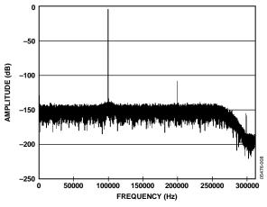
Figure 15. Low Power FFT, 100 kHz, -0.5 dB Input Tone, 32× Decimation
