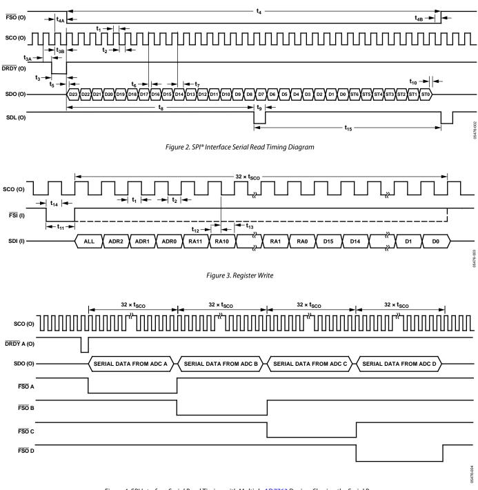
Figure 4. SPI Interface Serial Read Timing with Multiple AD7763 Devices Sharing the Serial Bus
