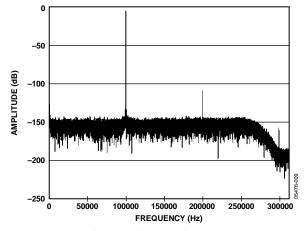
Figure 12. Normal Mode FFT, 100 kHz, -0.5 dB Input Tone, 32× Decimation
