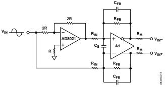
Figure 33. Single-Ended-to-Differential Conversion
