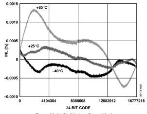
Figure 22. 24-Bit INL, Low Power Mode
