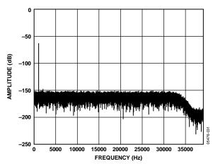
Figure 10. Low Power FFT, 1 kHz, –6 dB Input Tone, 256× Decimation
