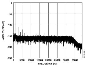
Figure 9. Low Power FFT, 1 kHz, -0.5 dB Input Tone, 256× Decimation
