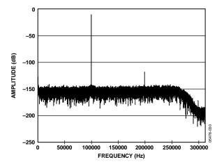
Figure 13. Normal Mode FFT, 100 kHz, –6 dB Input Tone, 32× Decimation
