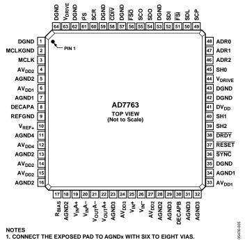
Figure 5. Pin Configuration
