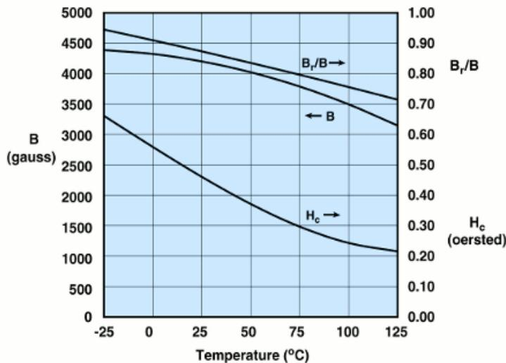
Measured on a 13/8/6mm toroid at 10 kHz. B is measured at H=10 oersted.
