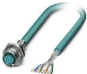
Bus system flush-type socket, Ethernet, 8-pos., M12, shielded, rear/screw mounting with M16 thread, with 1 m bus cable, 4 x 2 x 0.26 mm 2
