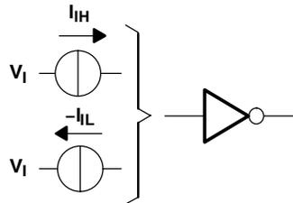
Figure 2. Driver Test Circuit for  $I_{IH}$  and  $I_{IL}$
