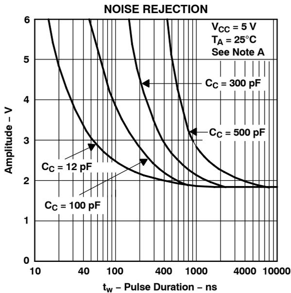
NOTE A: This figure shows the maximum amplitude of a positive-going pulse that, starting from 0 V, will not cause a change in the output level.
