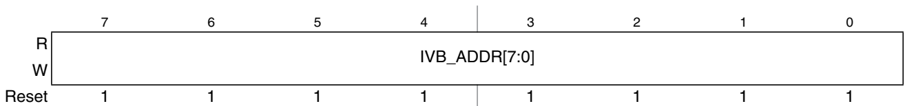
Figure 7-2. Interrupt Vector Base Register (IVBR)
