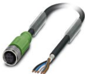
Sensor/actuator cable, 5-position, PUR halogen-free, black-gray RAL 7021, shielded, free cable end, on Socket straight M12, A-coded, cable length: 0.3 m
