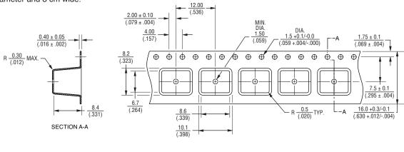
DIMENSIONS:  $\frac{\text{MM}}{(\text{INCHES})}$  Unless otherwise specified, tolerances in decimals are .X ± 0.3, .XX ± 0.15 for lengths in millimeters and ±1 ° for degrees.
