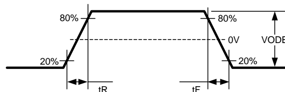
Figure 1. Driver Output Transition Time
