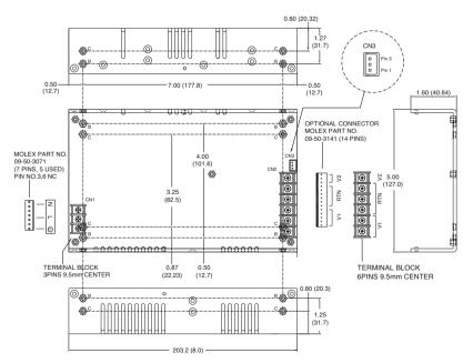
B: MOUNTING HOLE 8 PLACE 6-32 UNC(Zn-plated) SCALE 4:1
