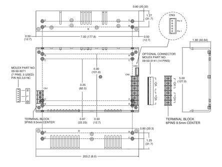
B: MOUNTING HOLE 8 PLACE 6-32 UNC(Zn-plated) SCALE 4:1
