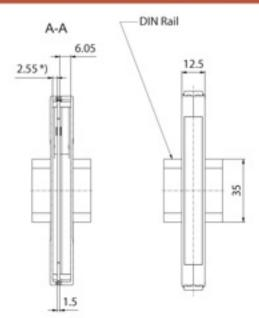
\*) 3.05 with printed circuit board thickness t = 1 mm
