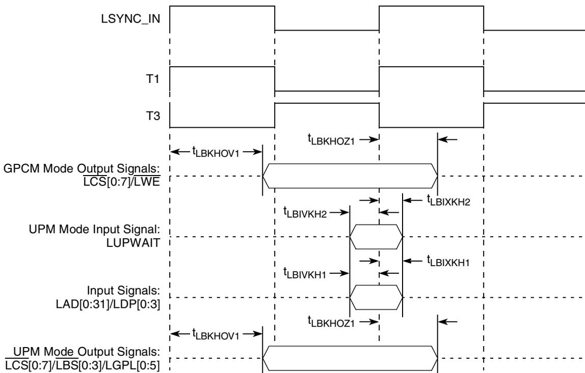
**Figure 19. Local Bus Signals, GPCM/UPM Signals for  $\text{LCCR}[\text{CLKDIV}] = 2$  (DLL Enabled)**
