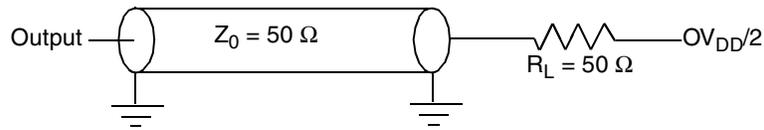
Figure 31. AC Test Load for the JTAG Interface
