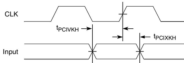
**Figure 39. PCI Input AC Timing Measurement Conditions**
