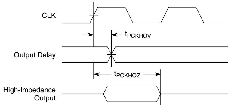
**Figure 40. PCI Output AC Timing Measurement Condition**
