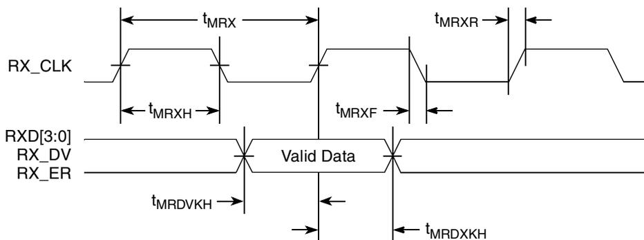
**Figure 11. MII Receive AC Timing Diagram**
