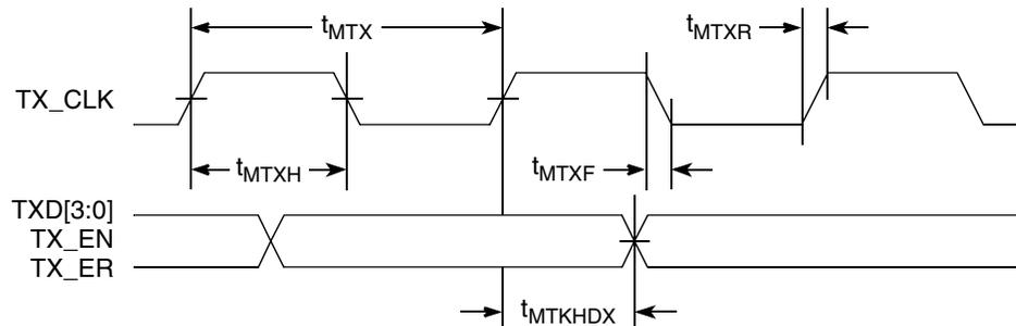
**Figure 10. MII Transmit AC Timing Diagram**
