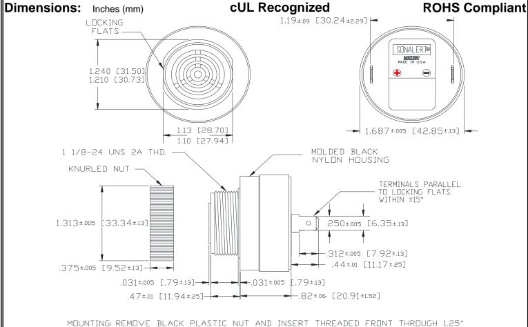
HOLE PUNCHED IN PANEL, IF ORIENTATION IS NEEDED, NOTE LOCKING FLATS
