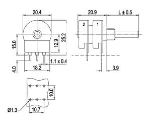
Dimensions are in millimeters and inches unless otherwise specified. Values in brackets are standard equivalents. Type 26 (Non Switched only)
