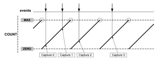
For input capture, the buffer register and the corresponding CCx act like a FIFO. When CCx is empty or read, any content in CCBx is transfered to CCx. The buffer valid flag is passed to set the CCx interrupt flag (IF) and generate the optional interrupt, event or DMA request.
