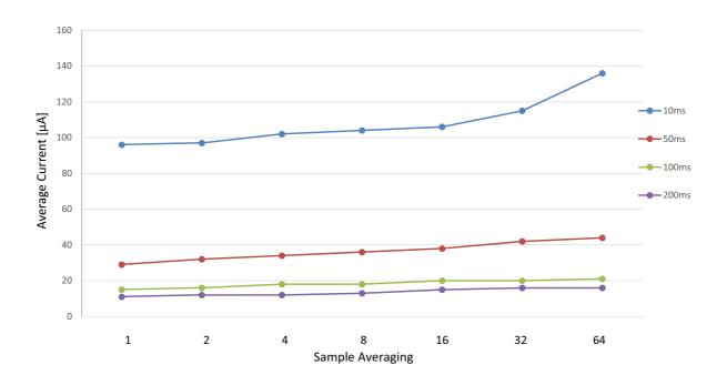
Figure 34-8. Power consumption [ $\mu$ A].
