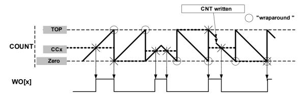
When MFRQ is used, the value in CC0 will be used as the top value and WO[0] will toggle on every overflow/underflow.
