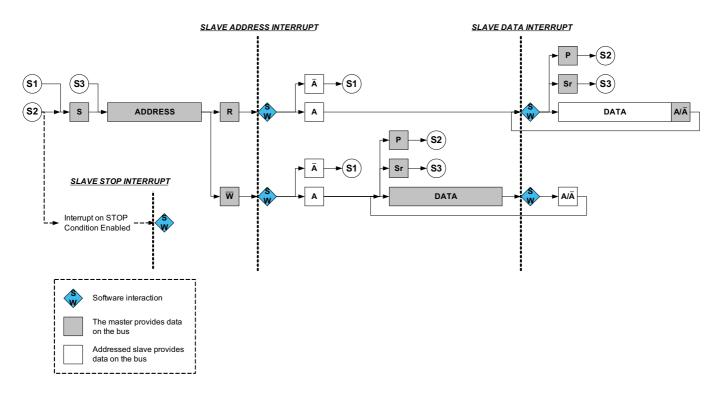
In the second strategy (SCLSM=1), interrupts only occur after the ACK bit as shown in Figure 27-11. This strategy can be used when it is not necessary to check DATA before acknowledging. For master reads, an address and data interrupt will be issued simultaneously after the address acknowledge, while for master writes, the first data interrupt will be seen after the first data byte has been received by the slave and the acknowledge bit has been sent to the master.
