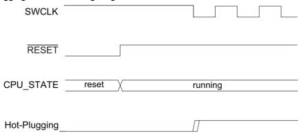
The presence of a debugger probe is detected when either Hot-Plugging or Cold-Plugging is detected. Once detected, the Debugger Present bit of the Status B register (STATUSB.DBGPRES) is set. For security reasons, Hot-Plugging is not available when the device is protected by the NVMCTRL security bit (refer to "Security Bit" on page 361).
