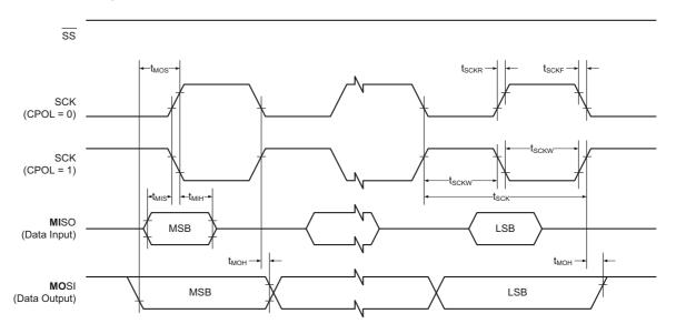
Figure 34-15.SPI timing requirements in slave mode
