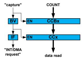
When the Capture x (MCx) bit and the buffer valid flag are set and a new capture event is detected, there is nowhere to store the new timestamp. In that case the Error bit in the Interrupt Flag Status and Clear register (INTFLAG.ERR) is set.
