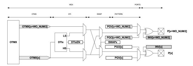
The output matrix (OTMX) unit distributes compare channels, according to the selectable configurations, as shown in Table 29-4.
