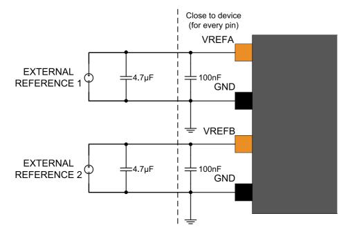
Figure 36-3. External Analog Reference Schematic With One Reference
