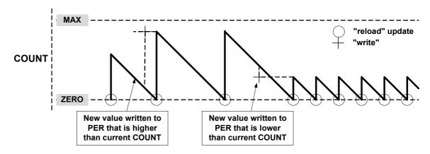
A counter wraparound can occur in any mode of operation when up-counting without buffering, as shown in Figure 29-11. This due to the fact that COUNT and TOP are continuously compared, and if a new value that is lower than the current COUNT is written to TOP, COUNT will wrap before a compare match happen.
