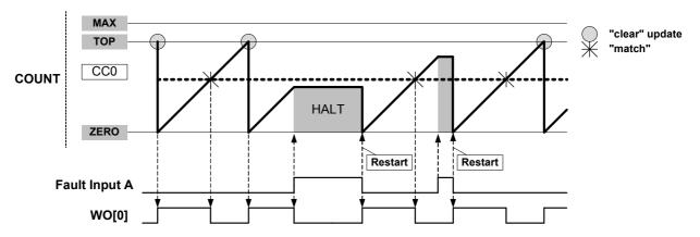
Figure 29-30. Waveform Generation with Fault Qualification, Halt and Restart Actions
