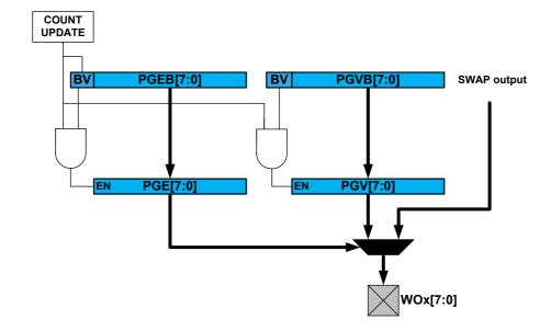
As with other double buffered timer/counter registers, the register update is synchronized to the UPDATE condition set by the timer/counter waveform generation operation. If the synchronization is not required by the application, the software can simply access directly the PATT.PGE, PATT.PGV bits registers.
