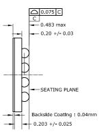
Notes: 1. Dimension "b" is measured at the maximum ball diameter in a plane to the seating plane.
