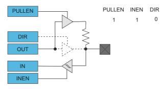
Note that when pull is enabled, the pull value is defined by the OUTx value.
