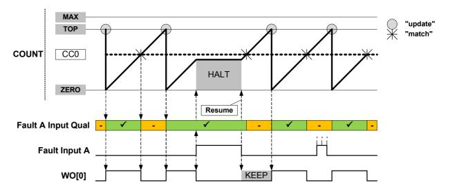
The software halt action can be configured using Faultn Halt mode bits in Recoverable Faultn
