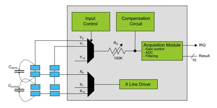
Figure 33-2. PTC Block Diagram Self-capacitance
