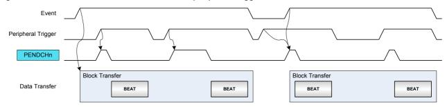
**Channel suspend:** When the channel suspend event action is selected, the event input is used to suspend an ongoing channel operation. The event is acknowledged when the current AHB access is completed. For further details on channel suspend, refer to "Channel Suspend" on page 284.
