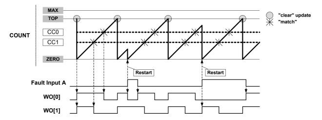
Figure 29-26. Waveform Generation in RAMP2 mode with Restart Action
