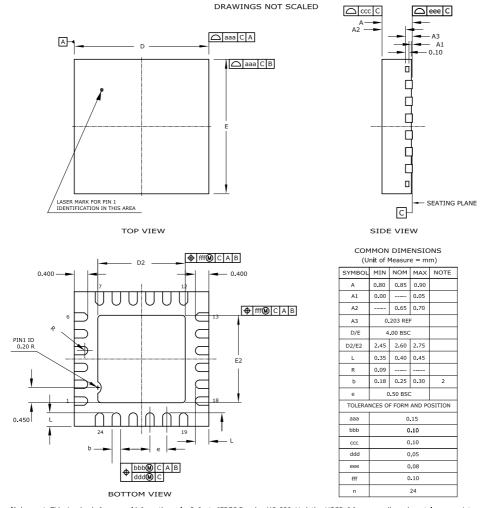
Notes: 1. This drawing is for general information only. Refer to JEDEC Drawing MO-220, Variation VGGD-6 for proper dimensions, tolerances, datums, etc. (excepted D2/E2 Min et Nom).
