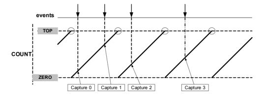
When the Capture Interrupt flag is set and a new capture event is detected, there is nowhere to store the new timestamp. As a result, the Error Interrupt flag in the Interrupt Flag Status and Clear register (INTFLAG.ERR) is set.
