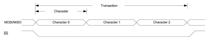
The SPI master must initiate a transaction by pulling low the slave select line  $(\overline{SS})$  of the desired slave. The master and slave prepare data to be sent in their respective shift registers, and the master generates the serial clock on the SCK line. Data are always shifted from master to slave on the master output, slave input line (MOSI), and from slave
