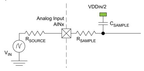
To achieve n bits of accuracy, the  $C_{SAMPLE}$  capacitor must be charged at least to a voltage of
