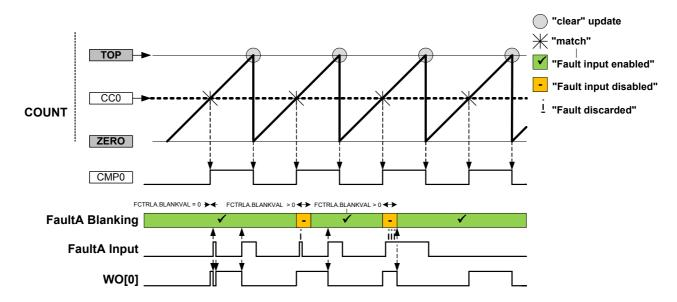
Fault Qualification can be enabled using Faultn Qualification bit in Recoverable Faultn Configuration register (FCTRLn.QUAL). When the recoverable fault qualification is enabled (FCTRLn.QUAL), the fault input is disabled all the time the corresponding channel output has an inactive level, as shown in Figure 29-22.
