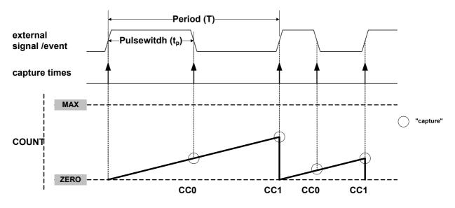
Selecting PWP or PPW in the Event Action bit group in the Event Control register (EVCTRL.EVACT1) enables the TCC to perform two capture actions, one on the rising edge and one on the falling edge.
