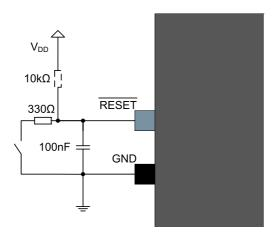
A pull-up resistor makes sure that the reset does not go low unintended causing a device reset. An additional resistor has been added in series with the switch to safely discharge the filtering capacitor, i.e. preventing a current surge when shorting the filtering capacitor which again causes a noise spike that can have a negative effect on the system.
