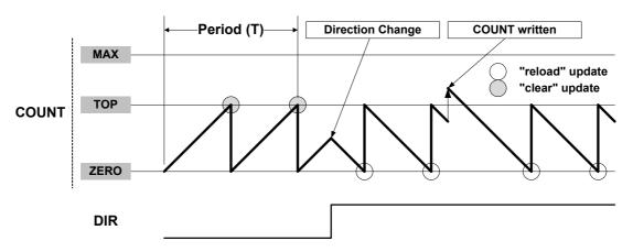
As shown in Figure 29-4, it is possible to change the counter value (by writing directly in the Count register) even when the counter is running. The write access has higher priority than count, clear, or reload. The direction of the counter can also be changed during normal operation. Due to asynchronous clock domains, the internal counter settings are written when the synchronization is complete.
