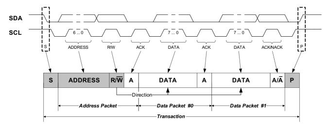
Figure 27-3. Transaction Diagram Syntax
