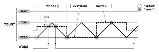
Using dual-slope PWM results in a lower maximum operation frequency compared to single-slope PWM generation.
