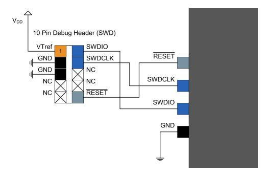
Table 36-8. Cortex Debug Connector (10-pin)
