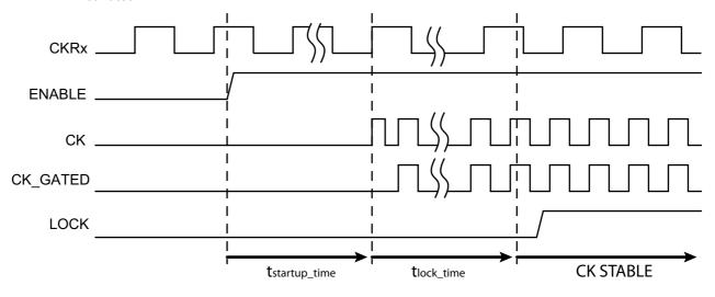
Figure 16-5. CK and CK\_GATED Output from Running Mode to FDPLL96M Off Mode
