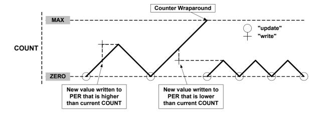
When double buffering is used, the buffer can be written at any time and the counter will still maintain correct operation. The period register is always updated on the update condition, as shown for dual-slope operation in Figure 29-14. This prevents wraparound and the generation of odd waveforms.
