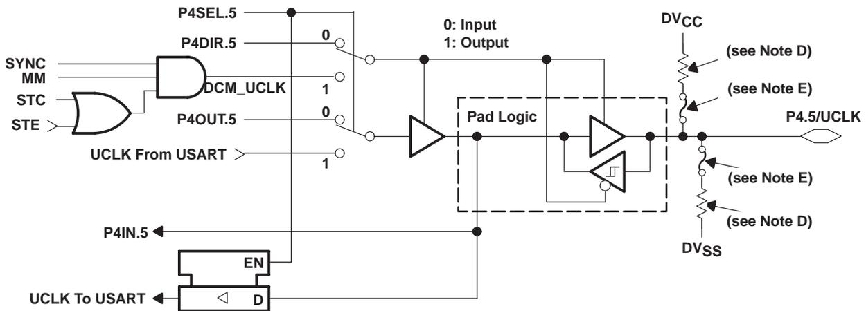
Figure 17. Port P4, P4.5, Input/Output With Schmitt-Trigger
