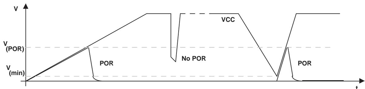
Figure 4. Power-On Reset (POR) vs Supply Voltage
