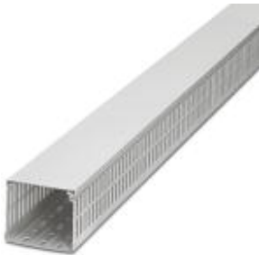
Cable duct, white, comprising upper part and mounting base, width: 40 mm, height: 100 mm, length: 2000 mm
