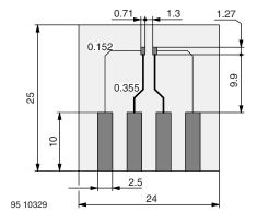
Fig. 3 - Board for R<sub>thJA</sub> Definition (in mm)
