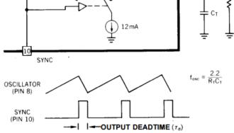
Figure 4. Oscillator Circuit
