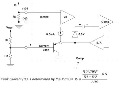
Figure 8. Pulse by Pulse Current Limiting
