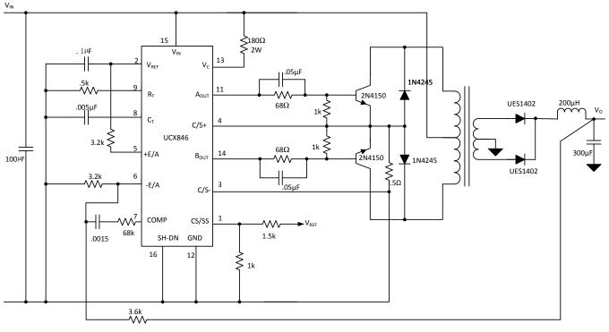
Figure 5. Typical Application Diagram
