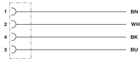
Contact assignment of the M12 socket
