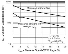
Fig. 4 - Typical Junction Capacitance
