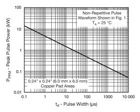
Fig. 2 - Peak Pulse Power Rating Curve
