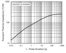
Fig. 6 - Typical Transient Thermal Impedance
