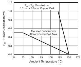
Fig. 5 - Power Dissipation Derating Curve
