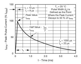
Fig. 1 - Pulse Waveform
