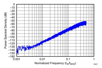
Figure 24. Modulator Noise Spectrum Up To 0.5 x f<sub>MOD</sub>
