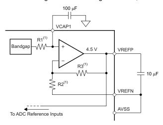
(1) For  $V_{REF} = 4.5 \text{ V}$ : R1 = 9.8 k $\Omega$ , R2 = 13.4 k $\Omega$ , and R3 = 36.85 k $\Omega$ .
