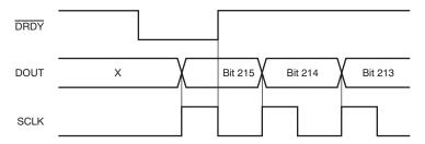
Figure 41.  $\overline{DRDY}$  with Data Retrieval ( $\overline{CS} = 0$ )
