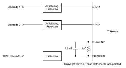
Figure 68. Setting Common-Mode Using BIAS Electrode
