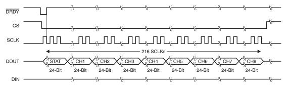
Figure 45. SPI Bus Data Output
