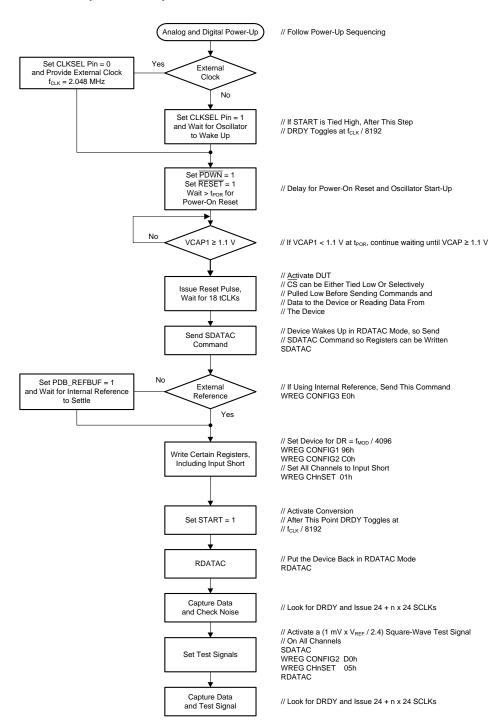
Figure 67. Initial Flow at Power-Up
