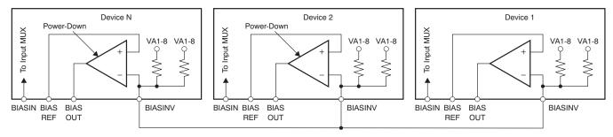
Figure 39. BIAS Drive Connection for Multiple Devices
