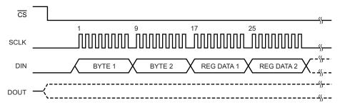
Figure 49. WREG Command Example: Write Two Registers Starting from 00h (ID Register) (BYTE 1 = 0100 0000, BYTE 2 = 0000 0001)
