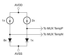
Figure 19. Temperature Sensor Measurement in the Input
