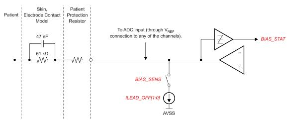
Figure 37. BIAS Lead-Off Detection at Power-Up
