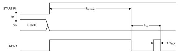
Figure 40. Settling Time
