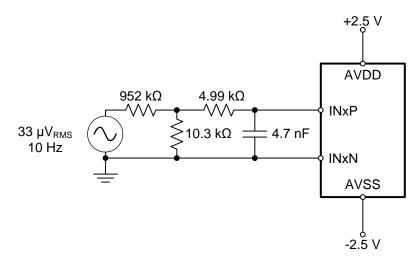
Figure 74. Example Schematic Using the ADS1299 in an EEG Data Acquisition Application, Referential Montage
