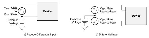
Figure 20. Methods of Driving the ADS1299-x: Pseudo-Differential or Fully Differential
