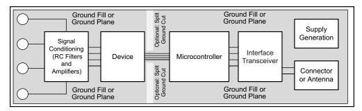
Figure 79. System Component Placement
