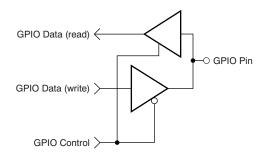
Figure 32. GPIO Port Pin
