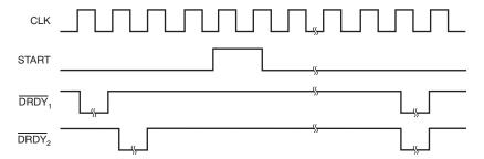
Figure 69. Synchronizing Multiple Converters
