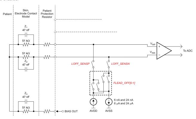
Figure 35. Lead-Off Detection
