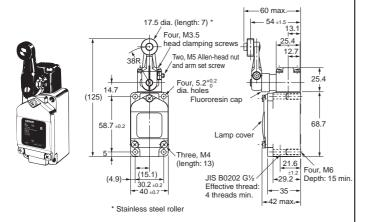
Roller Lever (Pre-wired connectors) WLCA2-\(\sigma\)-M1J\*/WL01\(\sigma\)-\(\sigma\)-M1J\* WLH2-\(\sigma\)-M1J\* WLGCA2-\(\sigma\)-M1J\*
