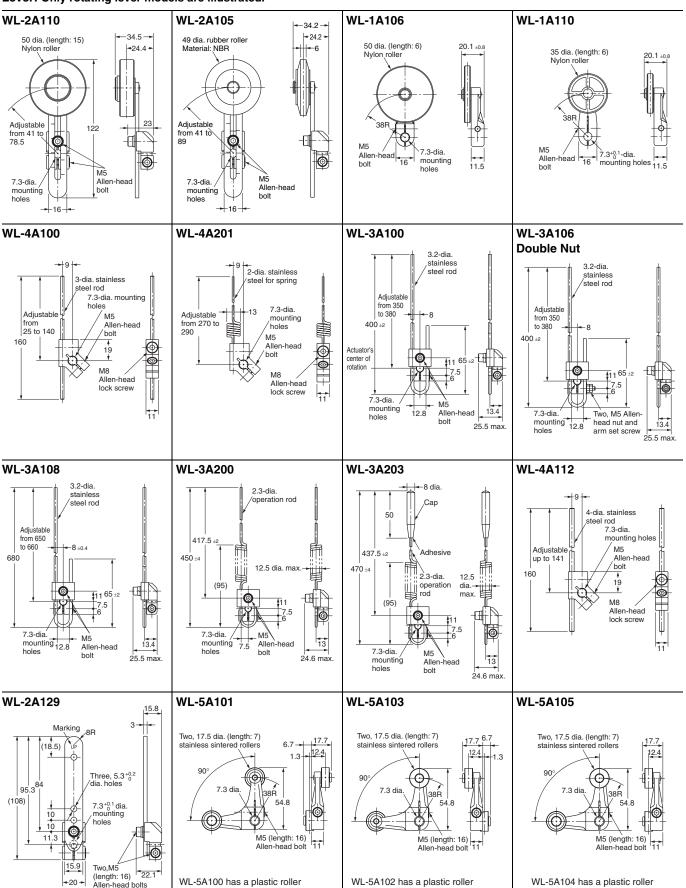
Note: 1. Unless otherwise indicated, a tolerance of  $\pm 0.4$  mm applies to all dimensions.
