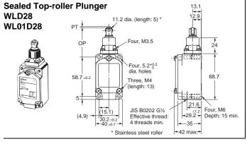
Note: Unless otherwise indicated, a tolerance of  $\pm 0.4~\text{mm}$  applies to all dimensions.
