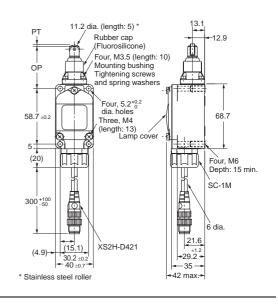
Note: Unless otherwise indicated, a tolerance of  $\pm 0.4 \ \text{mm}$  applies to all dimensions.
