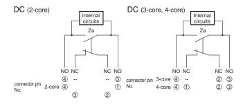
Note: Leakage current from indicator circuit may cause load's malfunction. Please check the load's OFF current before use the indicator-equipped switch.
