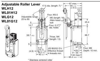
Note: 1. WL G12 is identical to other models except in the shape of the set position marker plate.
