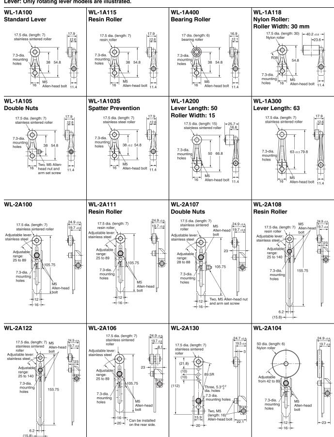
Note: Unless otherwise indicated, a tolerance of ±0.4 mm applies to all dimensions.
