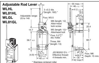
Note: 1. WL $\square$ GL is identical to other models except in the shape of the set position marker plate.
