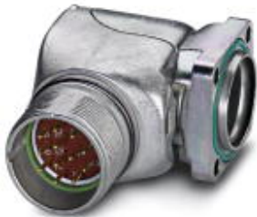
Device connector, front mounting, angled fixed, Screw locking, M23, number of positions: 12, type of contact: Pin, Crimp connection, Axial O-ring, 4x Ø 3.2, shielded: yes, flange dimensions: 26 mm x 26 mm
