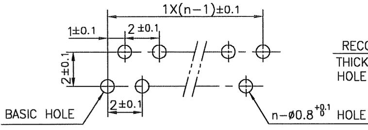
RECOMMENDED PC BOARD THICKNESS : 0.8~1.6 HOLE PATTERN (COMPONENT SIDE)
