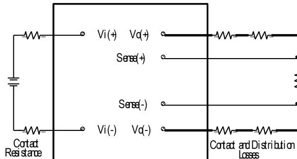
Figure 14: Effective circuit configuration for remote sense operation
