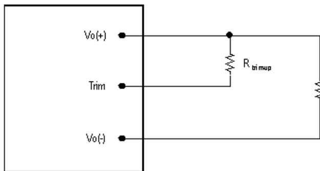
**Figure 16:** Circuit configuration for trim-up (increase output voltage)
