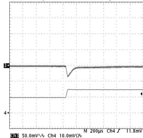
**Figure 6:** Output voltage response to step-change in load current (50%-75% of  $I_o$ , max;  $di/dt = 0.1A/\mu s$ ). Load cap:  $10\mu F$ ,  $100\ m\Omega$ ESR tantalum capacitor and  $1\mu F$  ceramic capacitor. Top Trace: Vout (50mV/div), Bottom Trace: Iout (5A/div).
