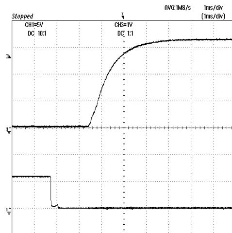
**Figure 4:** Turn-on transient at full rated load current (1 ms/div). Top Trace: Vout (1V/div); Bottom Trace: ON/OFF Control (5V/div).
