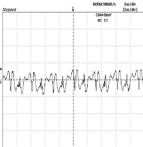
**Figure 9:** Input Reflected Ripple Current,  $i_S$ , at full rated output current and nominal input voltage with  $12\mu\text{H}$  source impedance and  $33\mu\text{F}$  electrolytic capacitor (2 mA/div).
