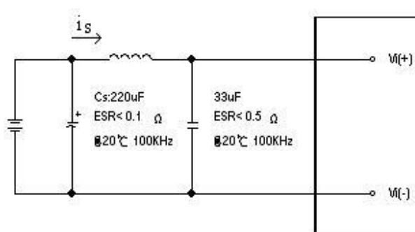
**Figure 8:** Test set-up diagram showing measurement points for Input Reflected Ripple Current (Figure 9). Note: Measured input reflected-ripple current with a simulated source Inductance ( $L_{TEST}$ ) of  $12\ \mu H$ . Capacitor  $C_s$  offset possible battery impedance.
