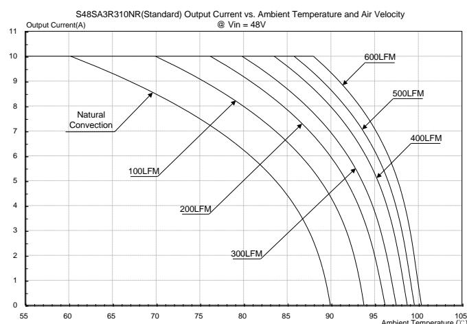
Figure 19: Output current vs. ambient temperature and air velocity @  $V_{in}=48V$
