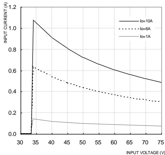
**Figure 3:** Typical input characteristics at room temperature.
