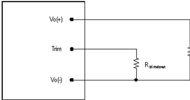
**Figure 15:** Circuit configuration for trim-down (decrease output voltage)
