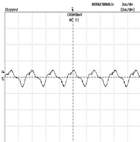
**Figure 11:** Output voltage ripple at nominal input voltage and rated load current (50 mV/div). Load capacitance:  $1\mu\text{F}$  ceramic capacitor and  $10\mu\text{F}$  tantalum capacitor. Bandwidth: 20 MHz.
