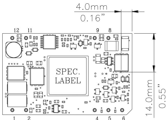
Figure 18: Hot spot temperature measured point
