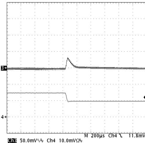
**Figure 7:** Output voltage response to step-change in load current (75%-50% of  $I_o$ , max;  $di/dt = 0.1A/\mu s$ ). Load cap:  $10\mu F$ ,  $100\ m\Omega$ ESR tantalum capacitor and  $1\mu F$  ceramic capacitor. Top Trace: Vout (50mV/div), Bottom Trace: Iout (5A/div).
