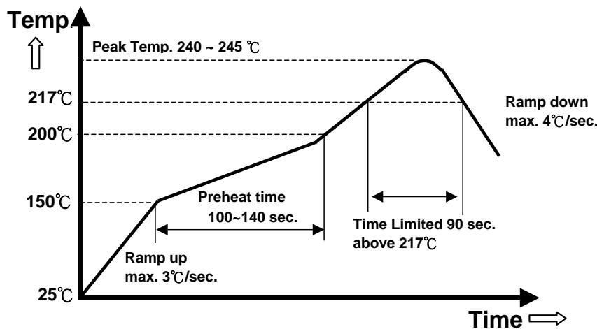
*Note: The temperature refers to the pin of S48SA, measured on the pin 1 (+Vout) joint.*
