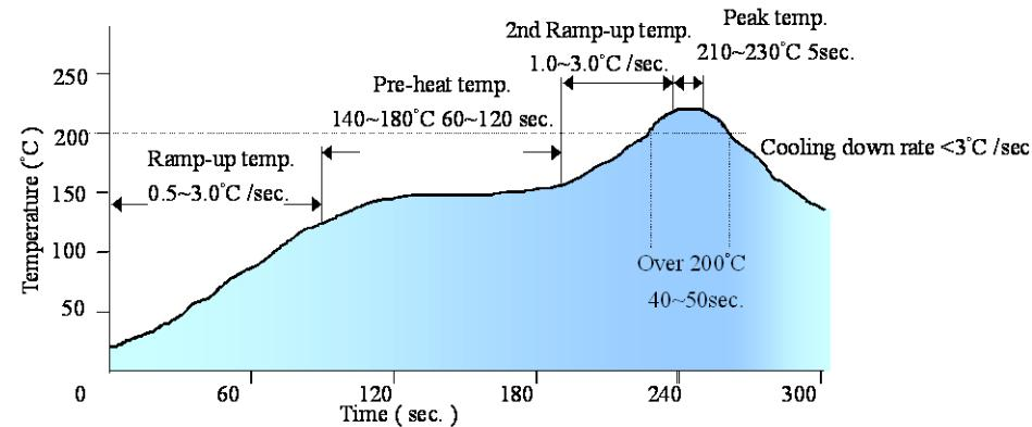
*Note: The temperature refers to the pin of S48SA, measured on the pin 1 (+Vout) joint.*
