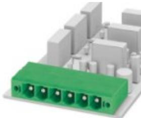
Header, Nominal current: 41 A, Rated voltage (III/2): 1000 V, Number of positions: 6, Pitch: 10.16 mm, Color: green, Contact surface: Silver, Mounting: Wave soldering, The nominal current of 76 A applies in connection with connectors from the PC 16 family. 41 A are reached in connection with PC 6 connectors (50 A in accordance with UL).
