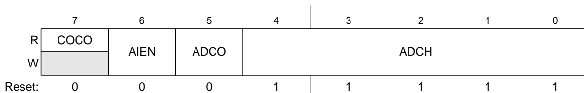
Figure 10-3. Status and Control Register (ADCSC1)
