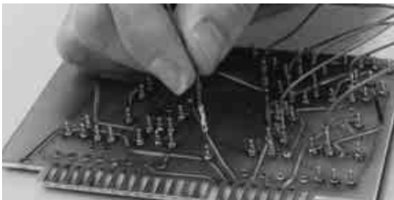
Printed Circuit Board Disconnects
