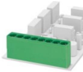
Header, Nominal current: 76 A, Rated voltage (III/2): 1000 V, Number of positions: 2, Pitch: 10.16 mm, Color: green, Contact surface: Silver, Mounting: Wave soldering, The nominal current of 76 A applies in connection with connectors from the PC 16 family. 41 A are reached in connection with PC 6 connectors (50 A in accordance with UL).
