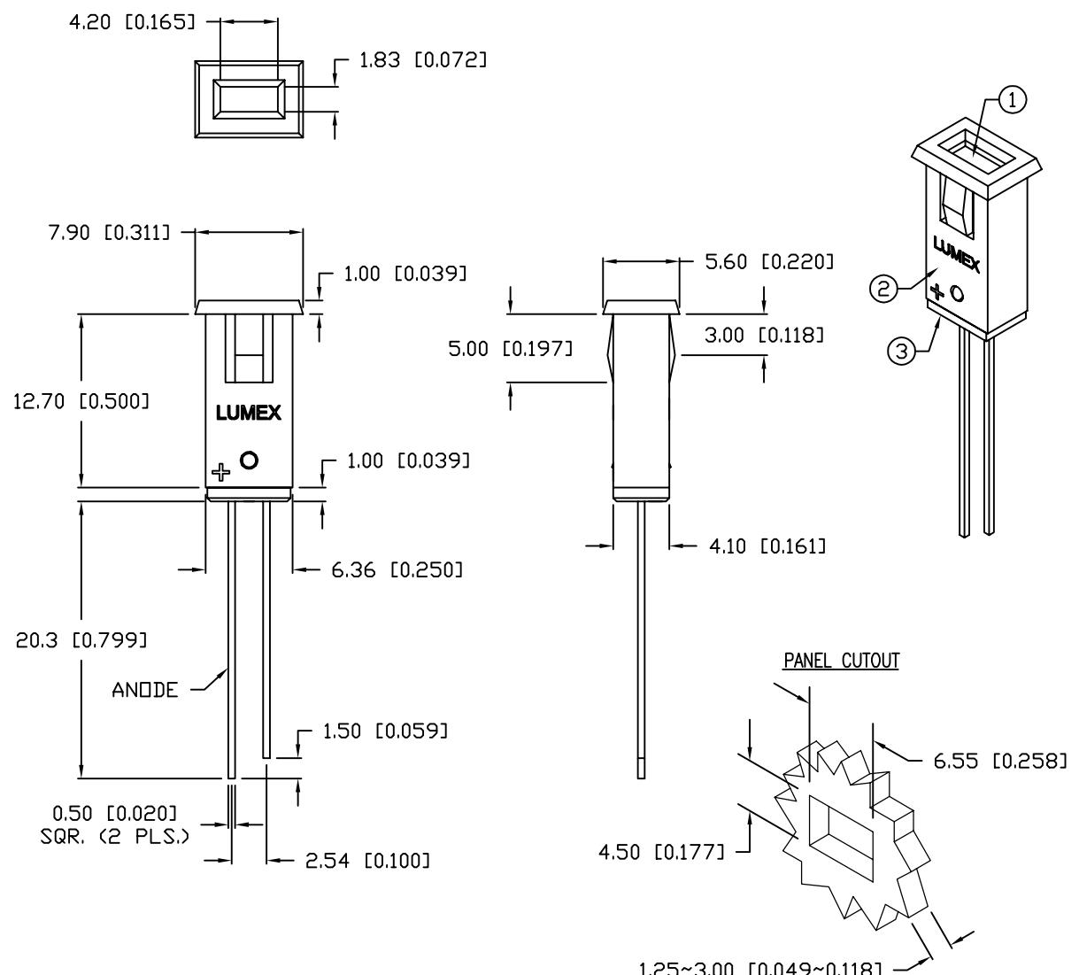
\*UNLESS OTHERWISE SPECIFIED TOLERANCES PER DECIMAL PRECISION ARE: X=±1 (±0.039), X.X=±0.5 (±0.020), X.XX=±0.25 (±0.010), X.XXX=±0.127 (±0.005). LEAD SIZE=±0.05 (±0.002), LEAD LENGTH=±0.75 (±0.030). MIN=  $^{+0.00}_{-0.00}$  DECIMAL PRECISION MAX=  $^{+0.00}_{-0.00}$  DECIMAL PRECISION
