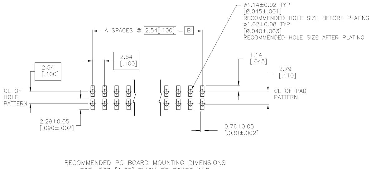
FOR .063 [1.60] THICK PC BOARD AND .012 [.305] STENCIL THICK.
