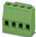
PCB terminal block, nominal current: 24 A, pitch: 5 mm, number of positions: 4, connection method: Screw connection with tension sleeve, mounting: Wave soldering, conductor/PCB connection direction: 0 °, color: green. Article with lateral pin exit
