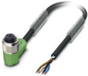
Sensor/actuator cable, 4-position, PUR halogen-free, black-gray RAL 7021, free cable end, on Socket angled M12, A-coded, cable length: 15 m
