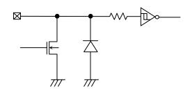
Figure 54. Input /output pin circuit diagram
