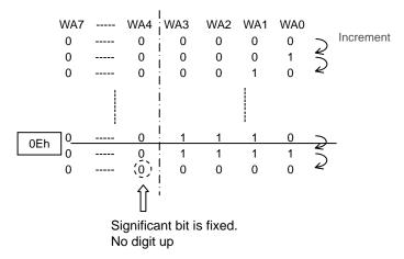
For example, when it is started from address 0Eh, therefore, increment is made as below, 0Eh→0Fh→00h→01h···, which please note. \* 0Eh···16 in hexadecimal, therefore, 00001110 becomes a binary number.
