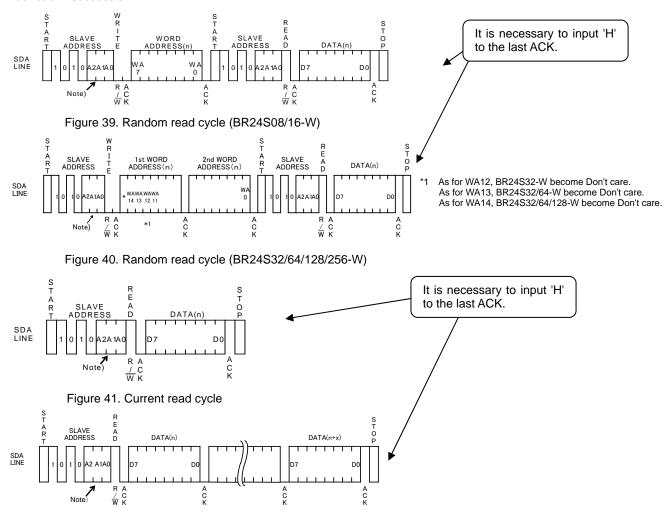
Figure 42. Sequential read cycle (in the case of current read cycle)
