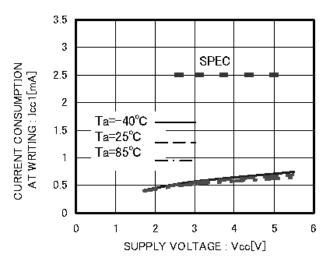
Figure 9. Current consumption at WRITE operation ICC1 (fscl=400kHz BR24S128/256-W)
