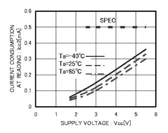
Figure 10. Current consumption at READ operation ICC2 (fscl=400kHz)
