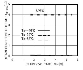
Figure 15. Start Condition Hold Time tHD:STA
