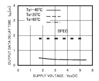
Figure 21. "L" Data output delay time tPD0
