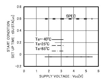
Figure 16. Start Condition Setup Time tSU:STA
