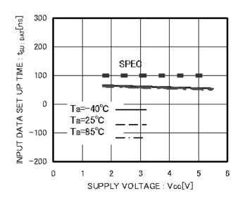
Figure 20. Input Data Setup Time tSU:DAT(LOW)
