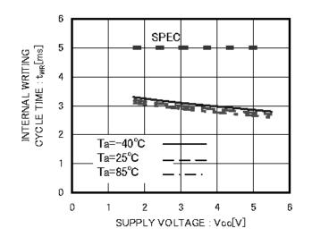
Figure 24. Internal writing cycle time tWR
