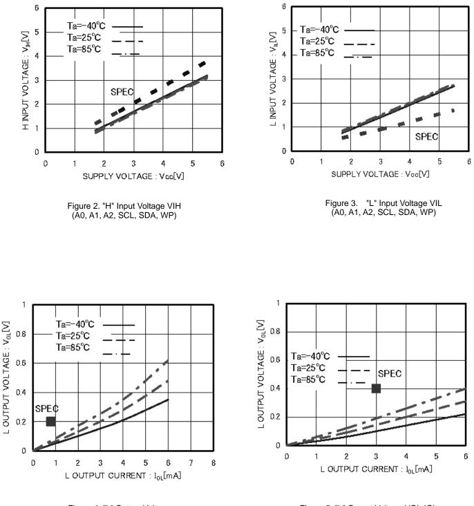
Figure 4. "L" Output Voltage VOL-IOL1(Vcc=1.7V)
