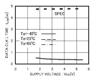
Figure 14. Data clock LOW Period tLOW
