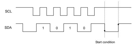
Figure 47. Case of cancel by start, stop condition during slave address input
