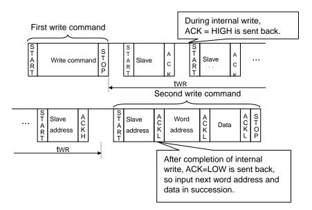
Figure 45. Case to continuously write by acknowledge polling
