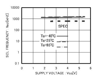
Figure 12. SCL frequency fSCL
