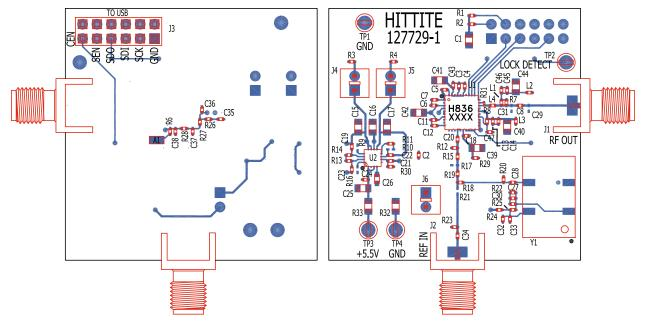
The circuit board used in the final application should use RF circuit design techniques. Signal lines should have 50 Ohm impedance while the package ground leads and exposed paddle should be connected directly to the ground plane similar to that shown. A sufficient number of via holes should be used to connect the top and bottom ground planes. The evaluation circuit board shown is available from Hittite upon request.
