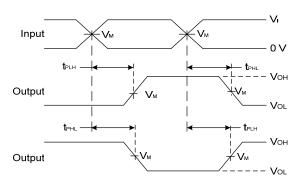
Voltage Waveform Propagation Delay Times
