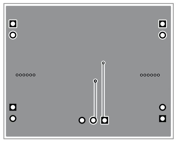
Figure 3. Bottom Layer Routing
