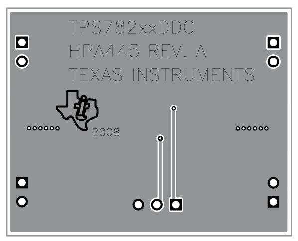
Figure 4. Bottom Layer Assembly
