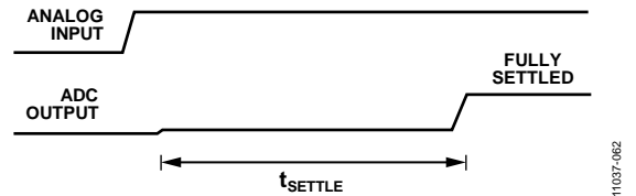
Figure 55. Step Input with Single Cycle Settling
