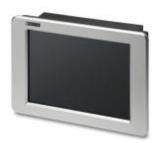
12.1"/30.7 cm flat panel LCD monitor with resistive touch screen. Includes two rear USB ports.
