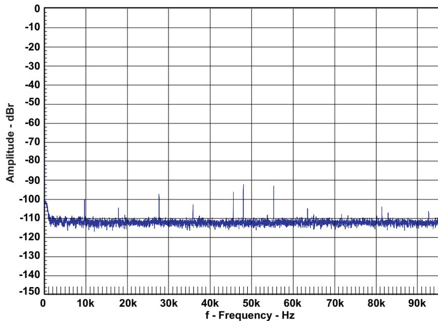
Figure 15. Idle Noise FFT Spectrum (Digital Input)
