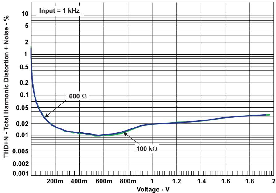
Figure 9. THD+N vs Voltage (Digital Input) Linear Scale
