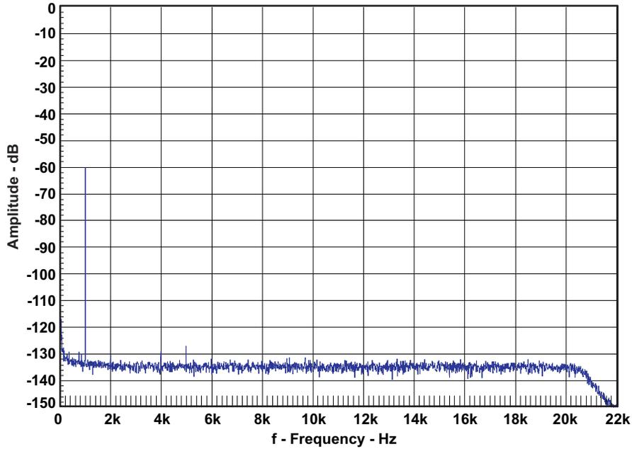
Figure 12. FFT Spectrum With -60-dBFS Tone (Analog Input)
