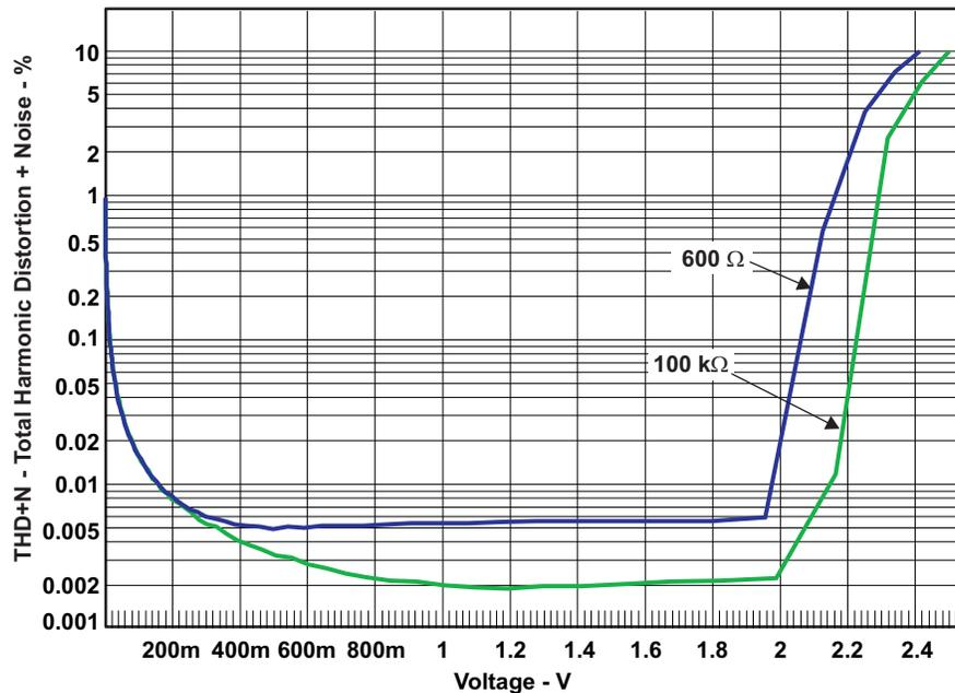
Figure 7. THD+N vs Voltage (Analog Input) Linear Scale
