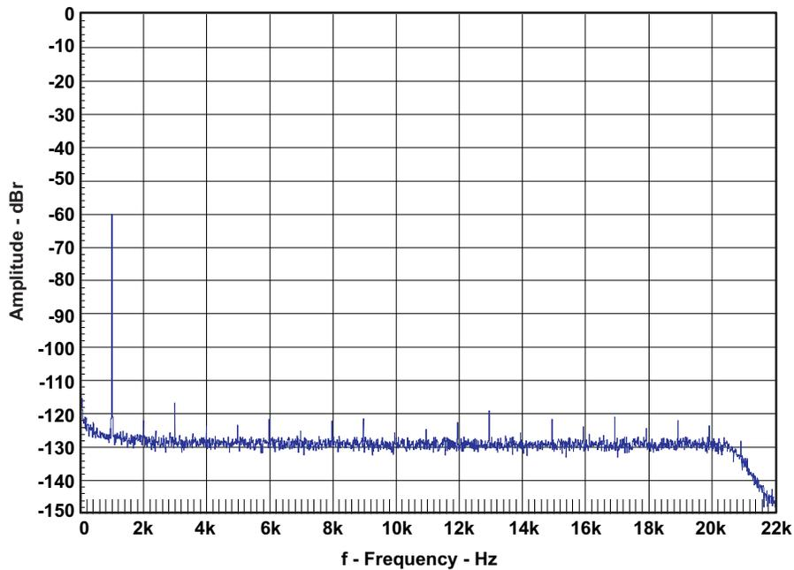
Figure 13. FFT Spectrum With -60-dBFS Tone (Digital Input)
