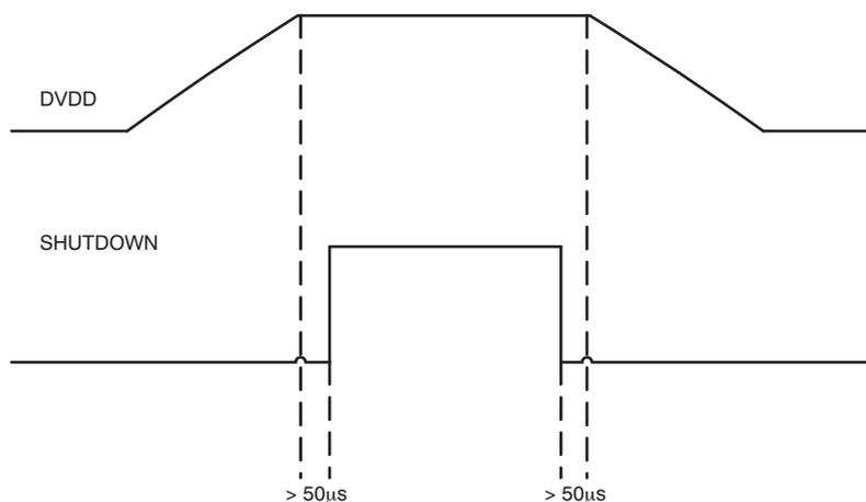
**Figure 4. Power-Up/Down Sequence**
