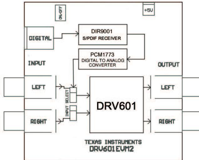
Figure 2. DRV601EVM2 Functional Block Diagram
