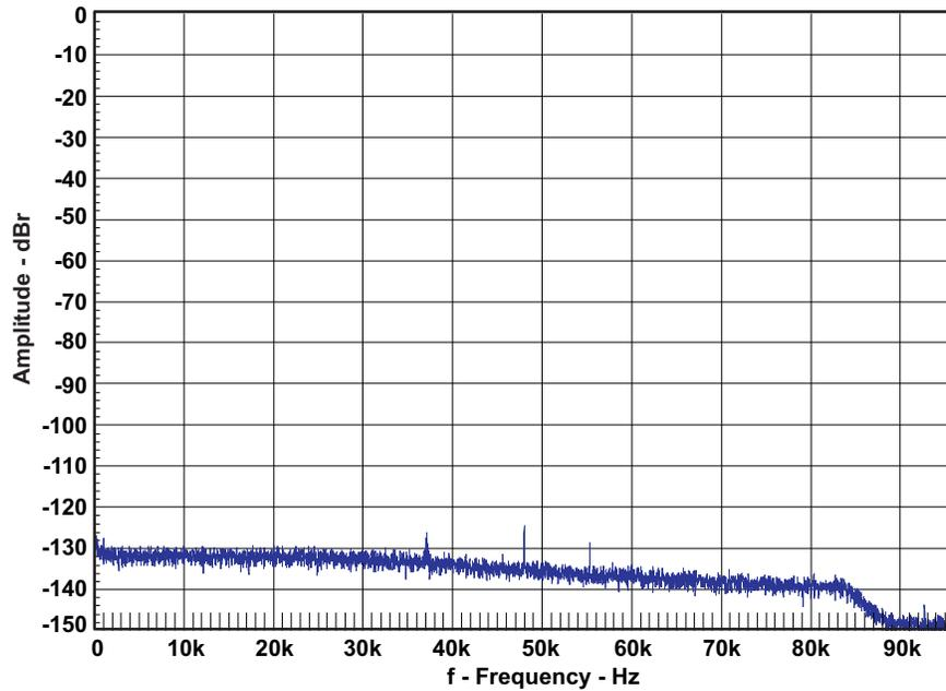
Figure 14. Idle Noise FFT Spectrum (Analog Input)
