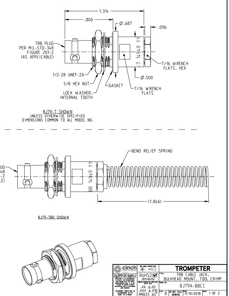
1.5 GASKET: SILICONE RUBBER 1.6 MOUNTING HARDWARE: NICKEL PLATED COPPER ALLOY 1.7 BEND RELIEF SPRING: PASSIVATED STAINLESS STEEL 2. ELEC TRICAL: 2.1 FREQUENCY (MAX): 500 MHz 2.2 IMPEDANCE: NON-CONSTANT 3. PANEL NUT TORQUE (MAX): 40 IN-LBS 4. ASSEMBLE PER TABLE 1. 5. EXAMPLE OF COMPLETE MODEL NO. BJ79 A -BB BR -BEND RELIEF SPRING (OPTIONAL) ASSEMBLY DASH NO. - KEYING LETTER PER TABLE 2 (AS APPLICABLE)
